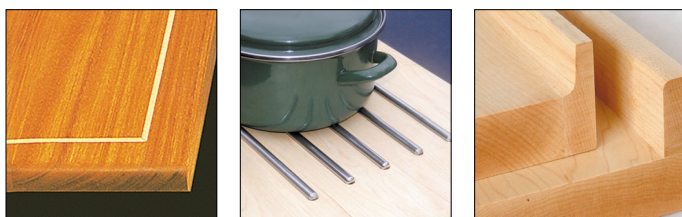
Fig 7. Stringing. Inset stringing in a contrasting timber - echoing other adjacent timbers perhaps.
